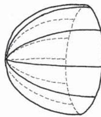
Surface is sliced into gores. Making the length of the gores equal to the circumference of the base gives a half-spherical shape.
