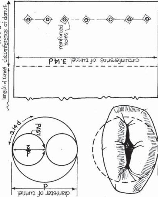
Hot Lips - a floppy donut at the end of a low pressure tunnel. When connected to the blower, small holes admit air to the tunnel from the lips, thereby inflating it.
